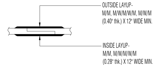
TYPICAL BODY JOINT DETAIL D NTS
