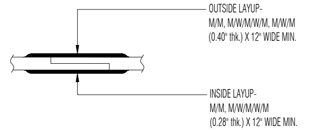
TYPICAL BODY JOINT DETAIL DETAIL D NTS
