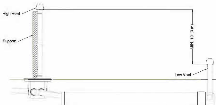
Figure 18. Example of Differential Venting for Gravity
