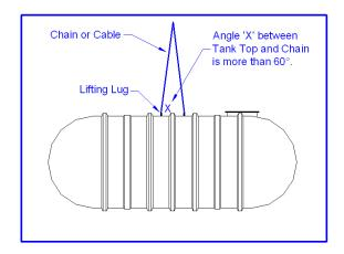
• *Do not* drop, impact, roll the tank or cause sudden stops while lifting the tank. Handle the tank with care.
